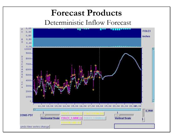
Each day CNRFC and DWR forecasters provide the Bureau of Reclamation with a 5-day forecast of both FNF and actual inflows to Folsom reservoir (6-hour time step). At low flow levels, reservoir releases produce a fluctuating inflow. Since we currently do not receive scheduled reservoir releases for the forecast period, the forecast hydrograph is based on the most recent reservoir release levels.
