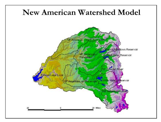
The new watershed model incorporates about 75% of the upstream storage in order to better forecast actual inflows into Folsom reservoir. Also inter-basin transfers within the Middle Fork and from the Middle Fork to the South Fork are accounted for and modeled in real-time.
