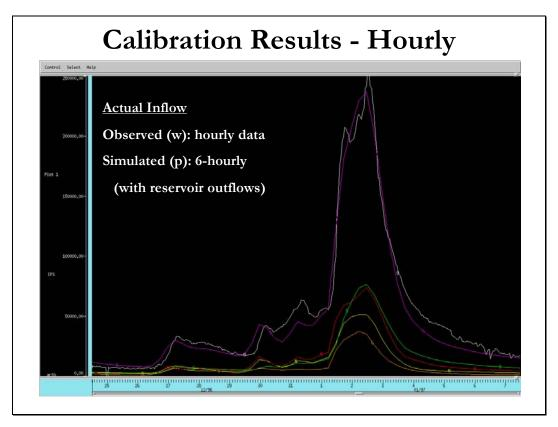
Hourly inflows to Folsom (in white) show three peaks. Assuming real-time knowledge of reservoir outflows, but no real-time gage data at NFDC1, MFAC1, and CBDC1, the simulated inflow remains close to the observed inflow both in volume and timing.
