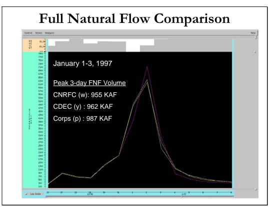
When calibrating the American watershed model, the goal was to simulate the full natural flow into Folsom as calculated by the DWR's California Data Exchange Center (CDEC). DWR's method of calculating the FNF is based on operational constraints, such that inflow into the upstream reservoirs is not routed down to Folsom. FNF calculations mirrored the daily calculations of the DWR. Differences in methodology can be seen in events where the inflows into upstream reservoirs are high.
