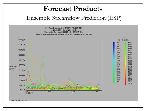
Ensemble products are also produced twice a week for reservoir operators. The "spaghetti plot" above presents the *conditional simulations* – simulations produced from historical precipitation and temperature record combined with the current soil and snow conditions.
