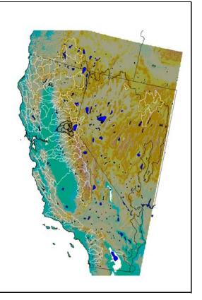
The California-Nevada River Forecast Center (CNRFC), together with the California Department of Water Resources (DWR), operates a continuous hydrologic model of the American River watershed. Each day the model is given real-time precipitation, temperature and flow data. The American River's nine sub-basins comprise only a small portion of the CNRFC's overall responsibility.
