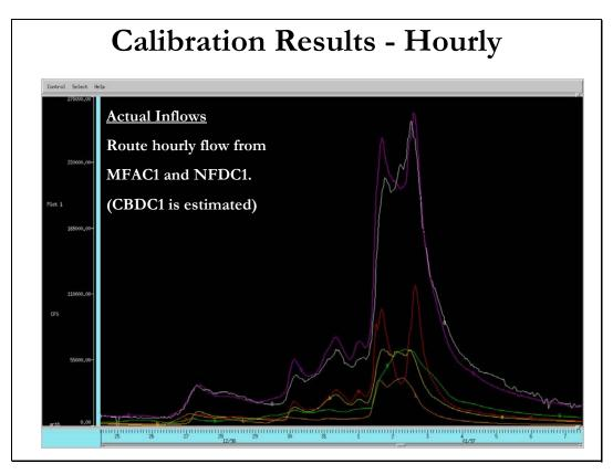
When real-time river gages are added to the model, more definition is added. Note: the gage at CBDC1 was washed out during the 1997 event. The flows used were based on estimations of daily flow at CBDC1.
